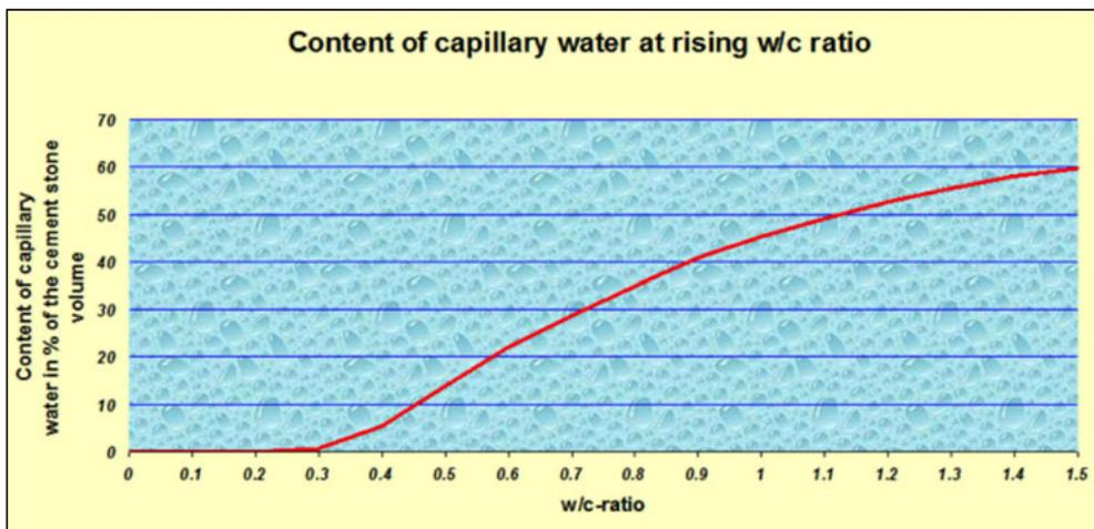
Two fold increase in capillaries from 0.5 to 0.6 W/C Ratio
